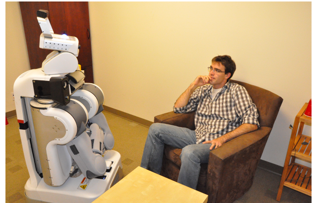
Figure 1. Personal Robot 2 asking the study participant for help with cleaning up the room (Study 2 lab environment strewn with empty cups). The small light on top of robot's head indicated the robot's source - autonomous, single teleoperator, or multiple teleoperators.
